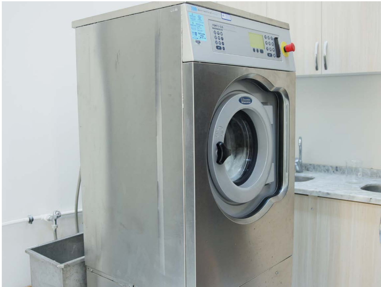
Wascator washing machine simulating domestic laundering, where full-sized clothes were washed
